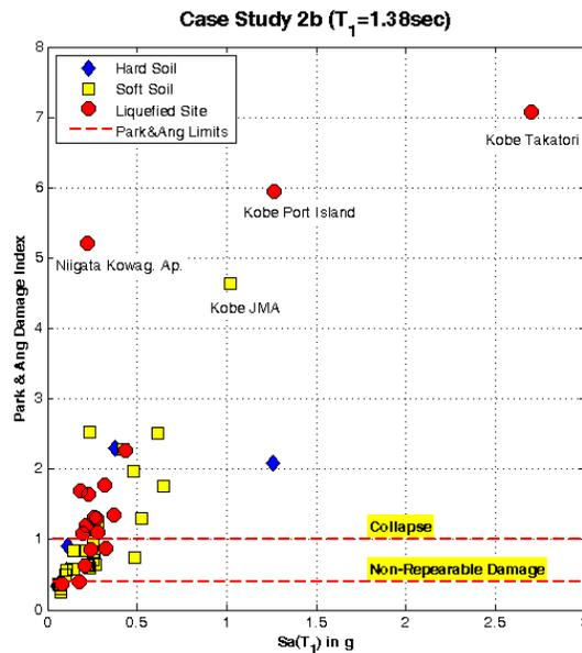
Figure 5. Comparison of the spectral acceleration at the fundamental period with the Park & Ang damage index for Case Study 2b ( $T_1=1.38$  s).
