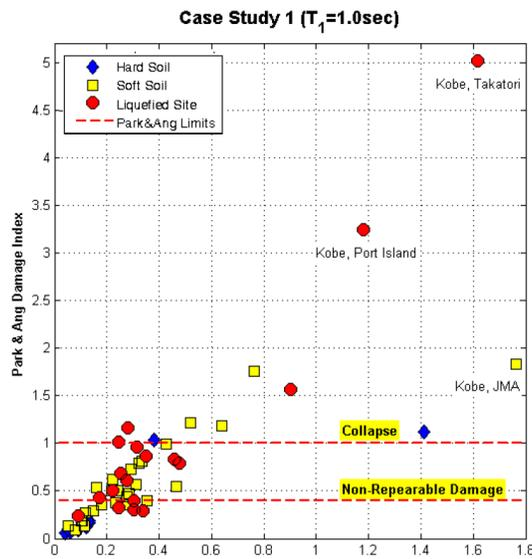
Figure 3. Comparison of the spectral acceleration at the fundamental period with the Park & Ang damage index for Case Study 1 ( $T_1 = 1.0$  s).
