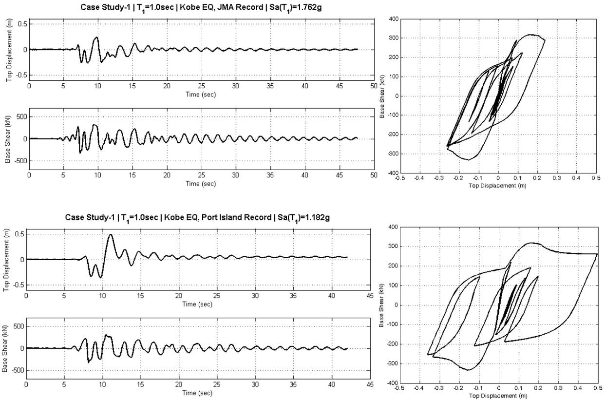
Figure 2. Base shear and top displacement response of case study 1 (top: JMA record w/o liquefaction, bottom: Port Island record w/ liquefaction)
