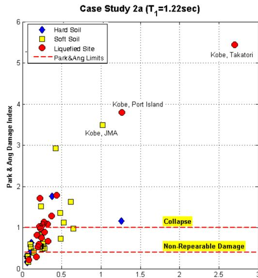
Figure 4. Comparison of the spectral acceleration at the fundamental period with the Park & Ang damage index for Case Study 2a ( $T_1=1.2$  s).
